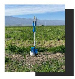
The Arbiter device includes multiple CO2 measurements to track carbon flux, and to monitor soil carbon respiration, and other agronomic indicators.
